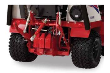
The Category One 3-Point Hitch adds the benefit of using numerous light and medium-duty implements\* on the rear of Ventrac 4520 Tractor. An eight-inch stroke hydraulic cylinder lifts up to 750 pounds (340 kg) at the draw bar through a 14 inch (26 cm) lift range. Each draft bar has a fast pin, adjustable stabilizing bar, and adjustable lift linkage.
